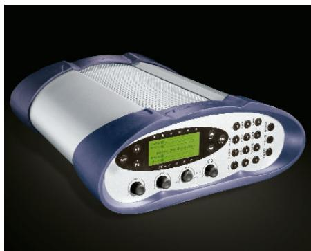
Let's start with the obvious application, the basic remote broadcast. Instead of lugging a mixer, a headphone amp, mic processing, a telephone and a codec I simply bring my mixer version Xstream. I send high-quality audio to the studios on one ISDN channel (the Xstream offers more coding modes than the Classic Zephyr and other ISDN codecs) and use the second channel to communicate with the studios.
