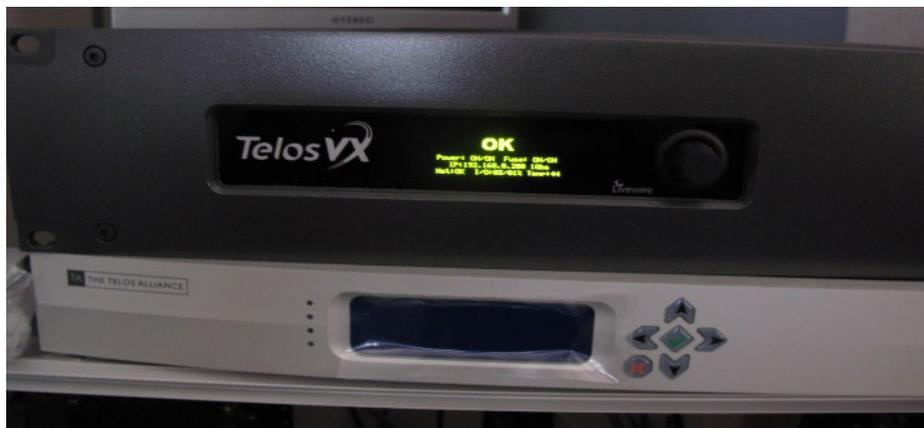
If you don’t see “The big OK”, there is an indication on the front panel and web GUI (system page) that will indicate what’s wrong. It’s usually a power supply not plugged powered, an ethernet not plugged in or the switch not set up for Livewire.
