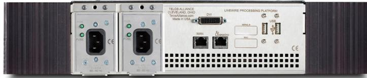
The VX Engine has two RJ-45 Ethernet jacks on the rear panel. Both are 100/1000 auto-speed and duplex setting. The (LAN) port is for Livewire audio and, by default, everything else, such as PCs used for web-based configuration, VSet phone controllers, producer PCs, and console controllers. This can be connected to an existing Livewire network or to a new, dedicated, network that you create to serve only the VX system, which could be as simple as a single Axia Approved Ethernet switch.
