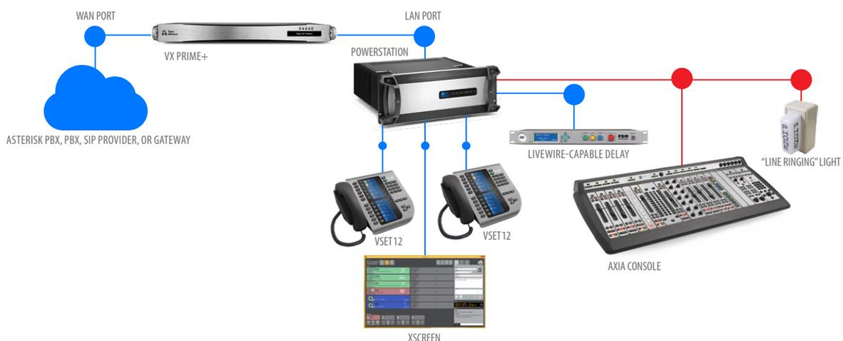
Installing a VX phone system in facilities already powered by Axia Livewire+™ AES67 networks requires even less time and hardware than described above. The audio inputs and outputs used and produced by VX are Livewire real-time audio channels and travel over the Axia AoIP network just like the rest of your audio. Axia console GPIO ports can be used for "phone ringing" tallies or remote control of profanity delay units.
