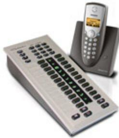
The call controller, along with a POTS telephone, emulates the functionality of the Desktop Director. It is suitable for any case where a reduced footprint, reduced complexity, or reduced cost is required.
