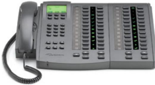
You have four columns in the Extended Director. In Talent mode, you can assign a caller to each of the four hybrids by pressing the corresponding button for that column. There is no need to use an Extended Director for Producer mode.
