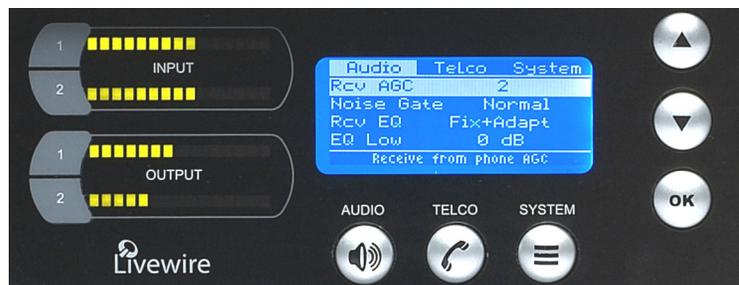
Pressing any menu button (**Audio**, **Telco**, or **System**) twice displays the Status screen.
