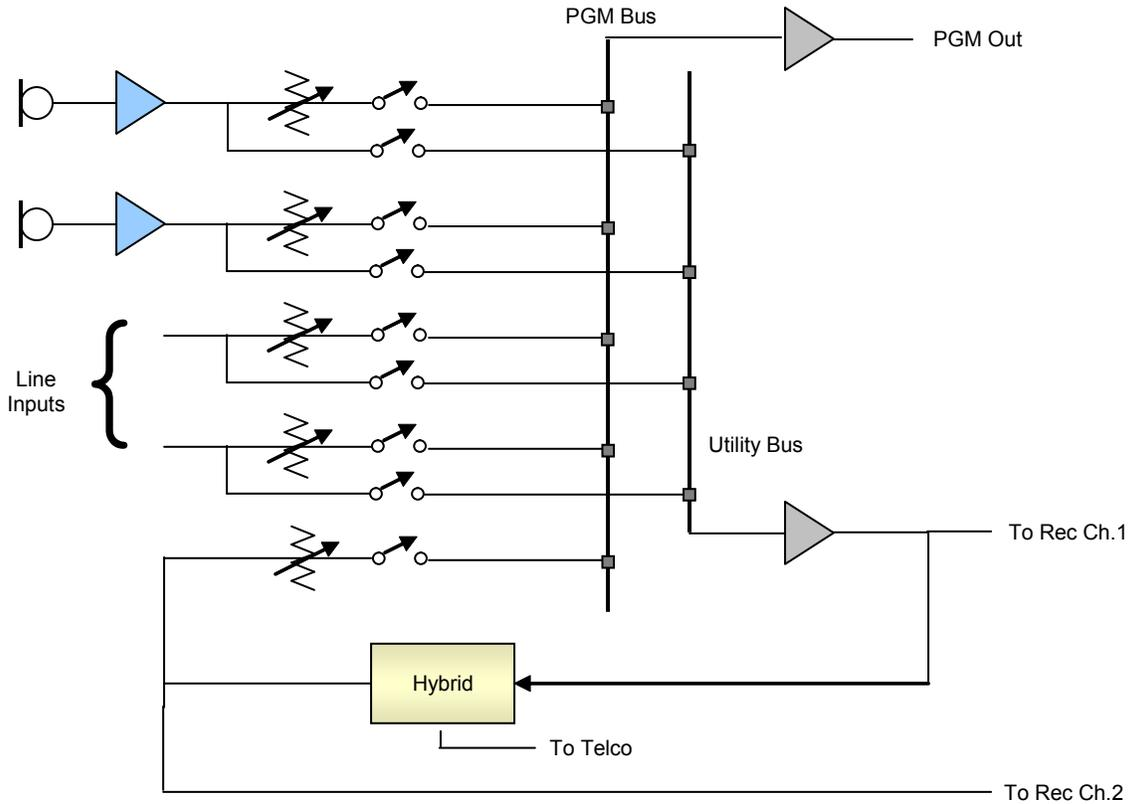
A recorder can be attached to the Utility and hybrid outputs to record announcer + phone audio. This is often done as shown here, with each signal to a separate track.
