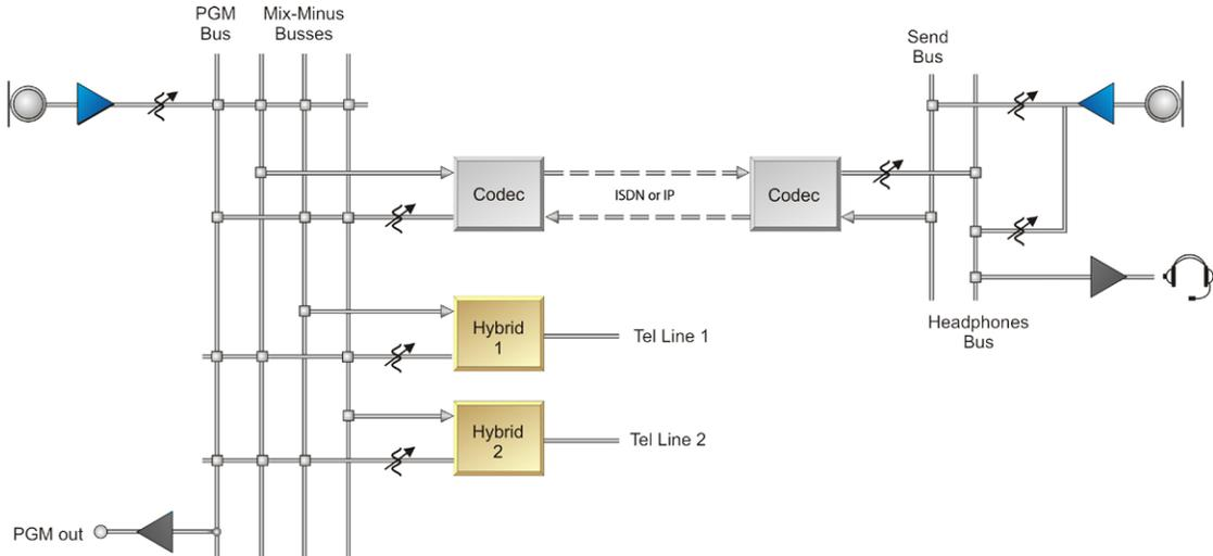
A problem could result from a hybrid with too much leakage and the codec delay. If the hybrid isn't doing a good job of preventing the send audio from leaking to its output, the remote mix-minus is corrupted. Remember, if any of the announcer audio from the remote site is returned, it will be delayed by the digital link, causing an echo effect in the announcer's headphones.
