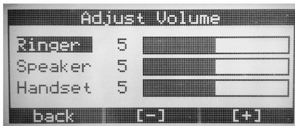
Press  $\Delta$  or  $\nabla$  to choose which level you want to adjust. Pressing [-] will decrease, while pressing [+] will increase the volume level for the item displayed. The change will take place immediately. Pressing the soft key button under the word **back** or the **Select** button will return you to the main screen. The following volume levels can each be individually adjusted:
