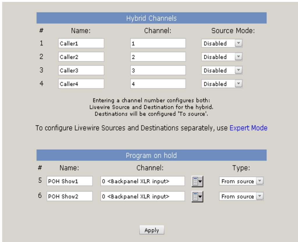
There are four hybrid channels. You can enter the Livewire text name and channel number or accept the defaults. Livewire channels are two-way, so this applies to both the send and receive audio. A Livewire enabled mixing console such as the Axia Element, when taking one of these as a source, will automatically connect both directions and provide the mix-minus. Cool, eh?
