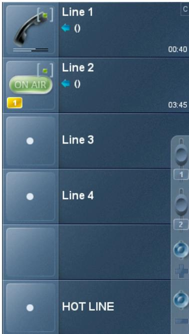
**TIME:** Each line will show length of time that has passed since the call has been on hold or ringing to the bottom right of the line field.
