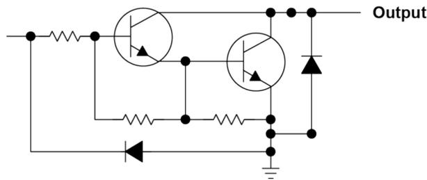
These will require a pull-up resistor to drive TTL-style logic inputs.
