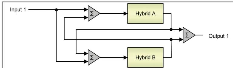
Its main purpose is to accommodate older consoles that have only one mix-minus and when only one fader is available for telephone calls. The disadvantage is that the operator has no control of the relative levels of the multiple callers. It relies upon the Hx6's AGC to automatically adjust the multiple callers to a consistent level.
