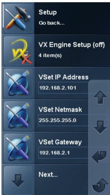
Press the 3 key (“VSet IP Address”) to edit the IP address.
