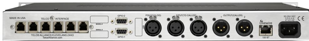
Output 1 is associated with Hybrid 1 audio. Output 2 is Hybrid 2 audio. Connect the output ports to your mixer or device you intend to use the Hx6 with. The XLR outs are standard active balance outs:
