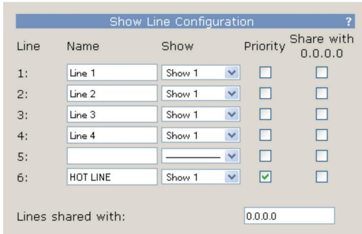
Line states can be shared with another Hx6. To do so, enter in the IP address of a second Hx6 and select which lines are shared. This is to be used when you splice an analog line between two Hx6 units. Both units require the opposing units IP address to be assigned in the IP field.
