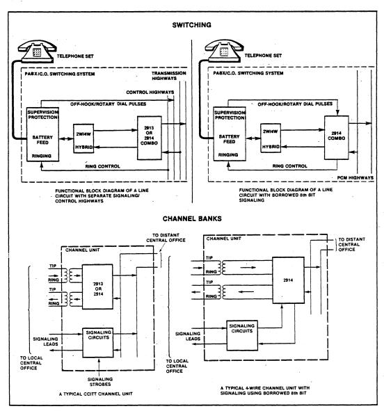
Figure 3. Typical Line Terminations
