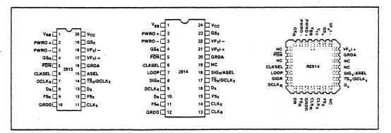
Figure 1. Pin Configurations
