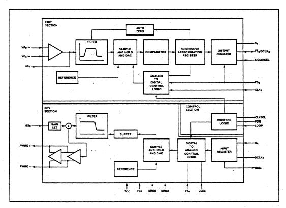
Figure 2 Block Diagram
