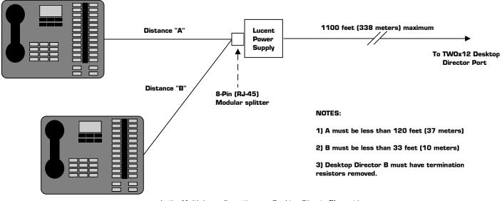
In the Multiple configuration one Desktop Director™ must be reconfigured to have its termination resistors removed (see below). This unterminated Desktop Director™ must be within 33 feet (10 meters) of the power supply Notes for Series 2101 User's.
