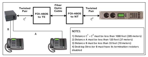
The above distance restrictions are theoretical values, based on the S interface specifications, and should work, assuming the fiber transceivers fully support the S interface standard. Telos has verified correct operation with the FOI-4605 in several configurations as follows:
