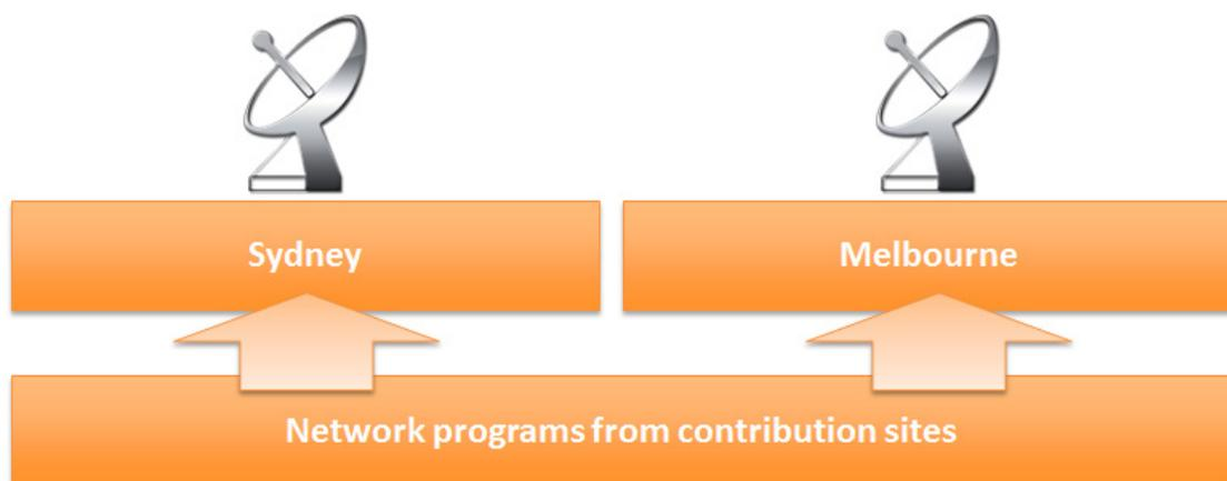
The selected uplink site radiates a DVB-S2 stream containing all of the audio streams onto the satellite. At the same time, the selected uplink site also presents these audio streams onto the SCA WAN for IGMP subscription. Using this method, a single uplink site is offering all network audio streams to the rest of the country using both satellite and WAN technologies. The second uplink site is receiving all audio streams and remains online as a "hot standby" for the current uplink site.
