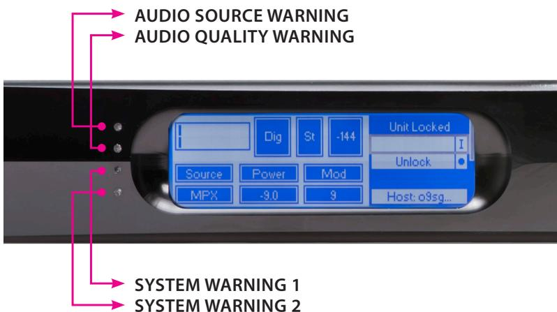
The top two LEDs denote audio conditions and alarms, the “Audio Source Warning” and “Audio Quality Warning” indicators. The bottom two are system status and alert indicators, “System Warning 1” and “System Warning 2”.
