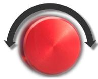
Rotating the wheel clockwise moves the highlighted selection on the LCD downward through menu options, or to the right through fields where you can enter numbers or text. When you're in one of those fields, the wheel scrolls through possible letters or numbers. Rotating it counter-clockwise does the reverse.
