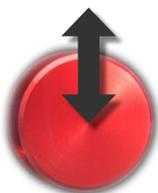
If you press the wheel in until it clicks, then quickly release it, the highlighted selection or field becomes active. This confirms a menu choice or option. If you do this in an entry field, you can then turn the wheel to select a value for that field. When an entry field shows the value you want, tap again to set it. Then the wheel returns to normal scrolling.
