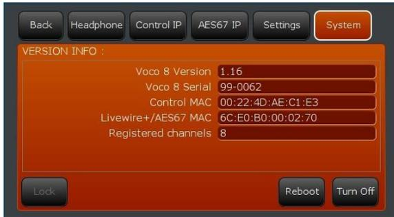
3. Verify the version currently loaded on your VOCO unit: Navigate to “More...System.” This update is intended for units running at least version 1.6. Insert the USB drive into the USB port on the front panel of your VOCO 8.
