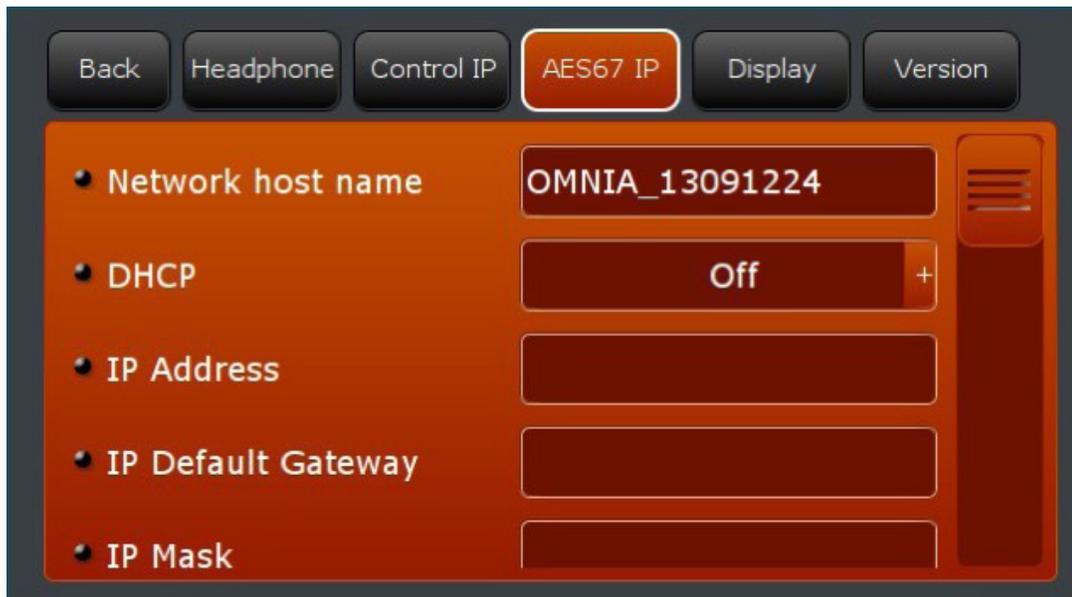
The screenshot shows a user interface for configuring the AES67 IP. At the top, there is a navigation bar with buttons for "Back", "Headphone", "Control IP", "AES67 IP" (which is highlighted in orange), "Display", and "Version". Below this, the configuration settings are listed on a dark orange background:
