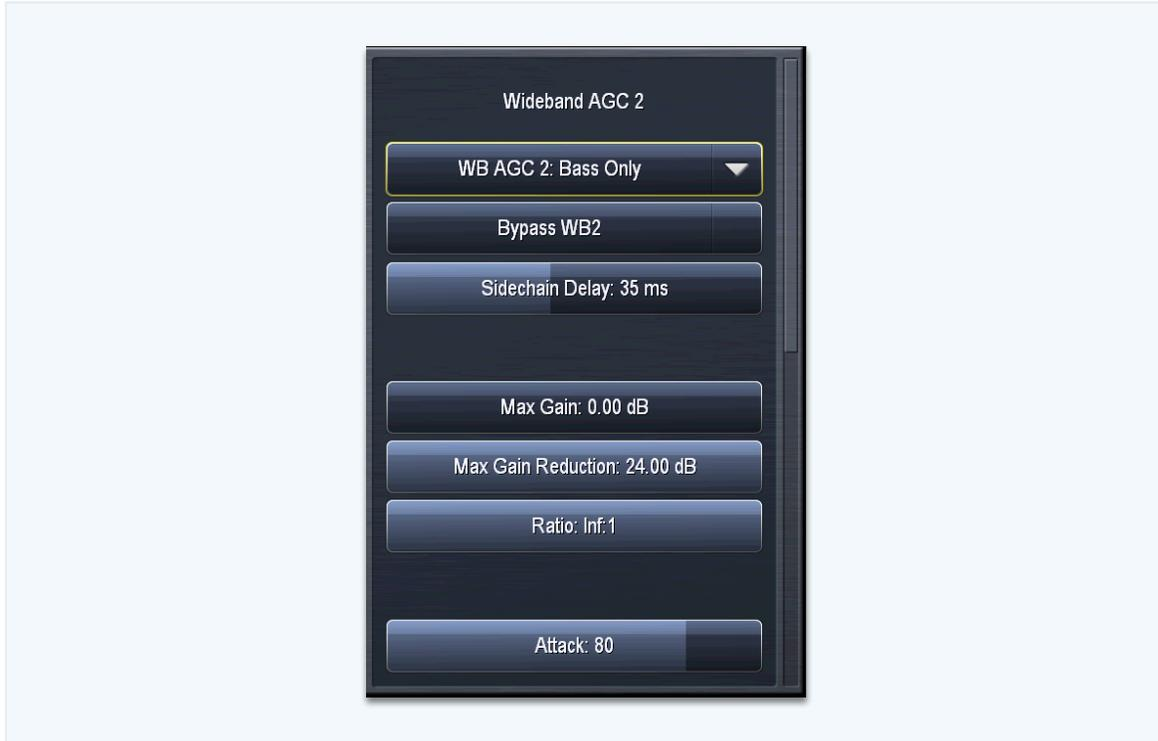
Multiband AGC's. This can be used as an additional wideband AGC or as a bass compressor.
