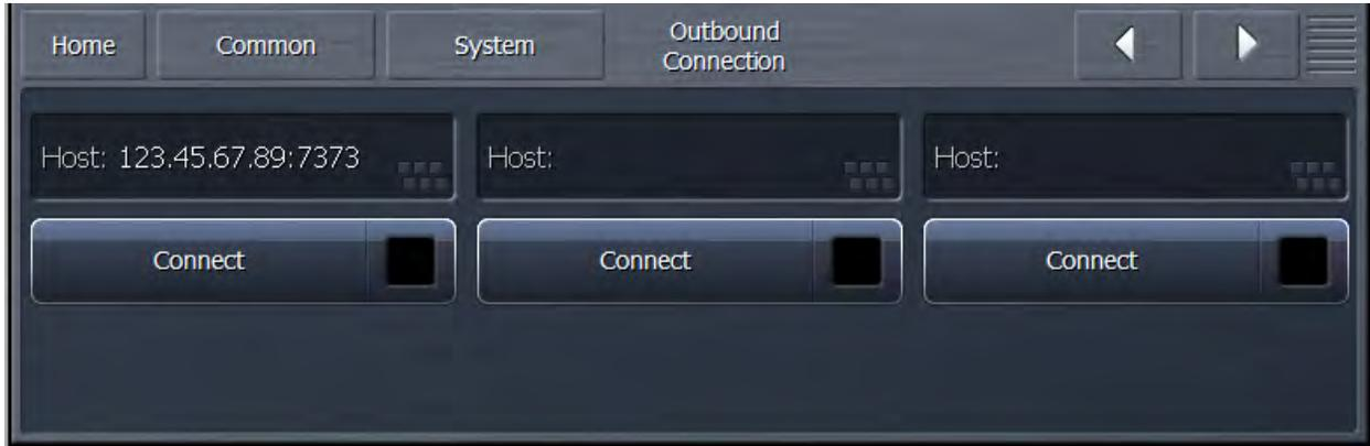
One example of how this can be used is for technical support. By creating an outbound connection, you are connecting to the support engineer's NfRemote computer which in turn allows them to control your Omnia.7.
