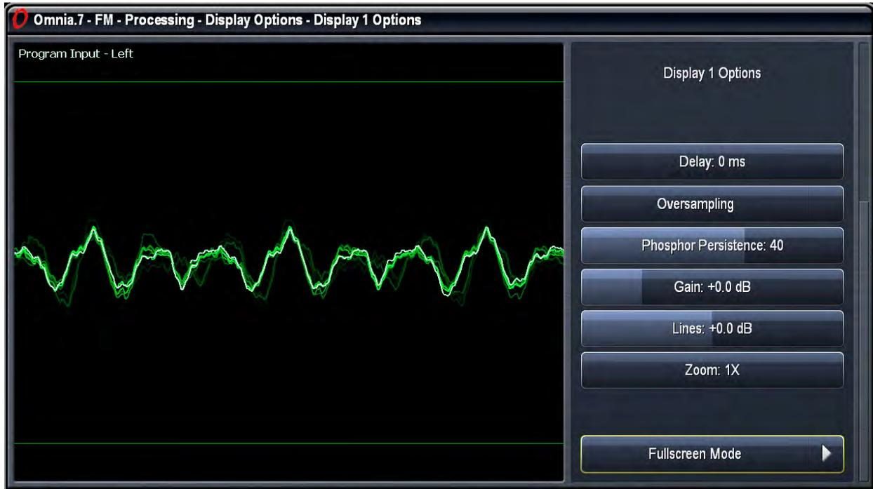
are provided in the Display Options menu. It may be necessary to scroll down to view these controls.
