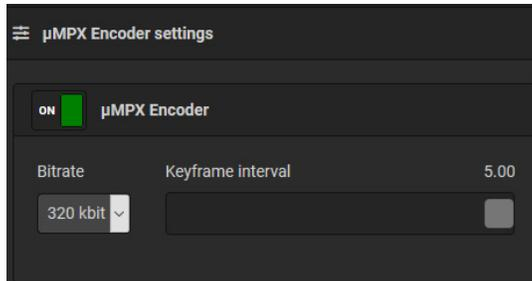
4. Set the bit rate you would like to transmit at (default is 320 kbps)
