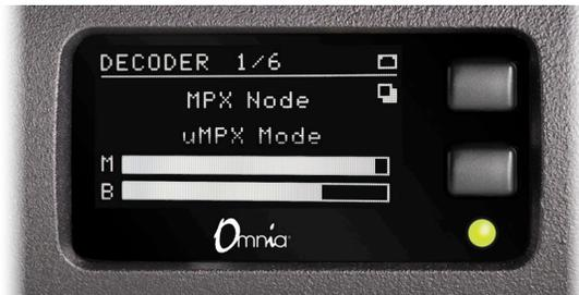
We recommend first configuring the Decoder on a test bench, as the output gain may need to be adjusted via dipswitch. By default, output is 4 volts, and 5 ohms.
