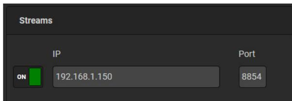
10. Connect to the target decoder if it is online and verify it is receiving the stream.
