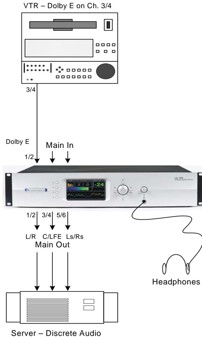
**Figure 3-8** LQ-1000 used for decode of Dolby E audio and loudness measurement during ingest
