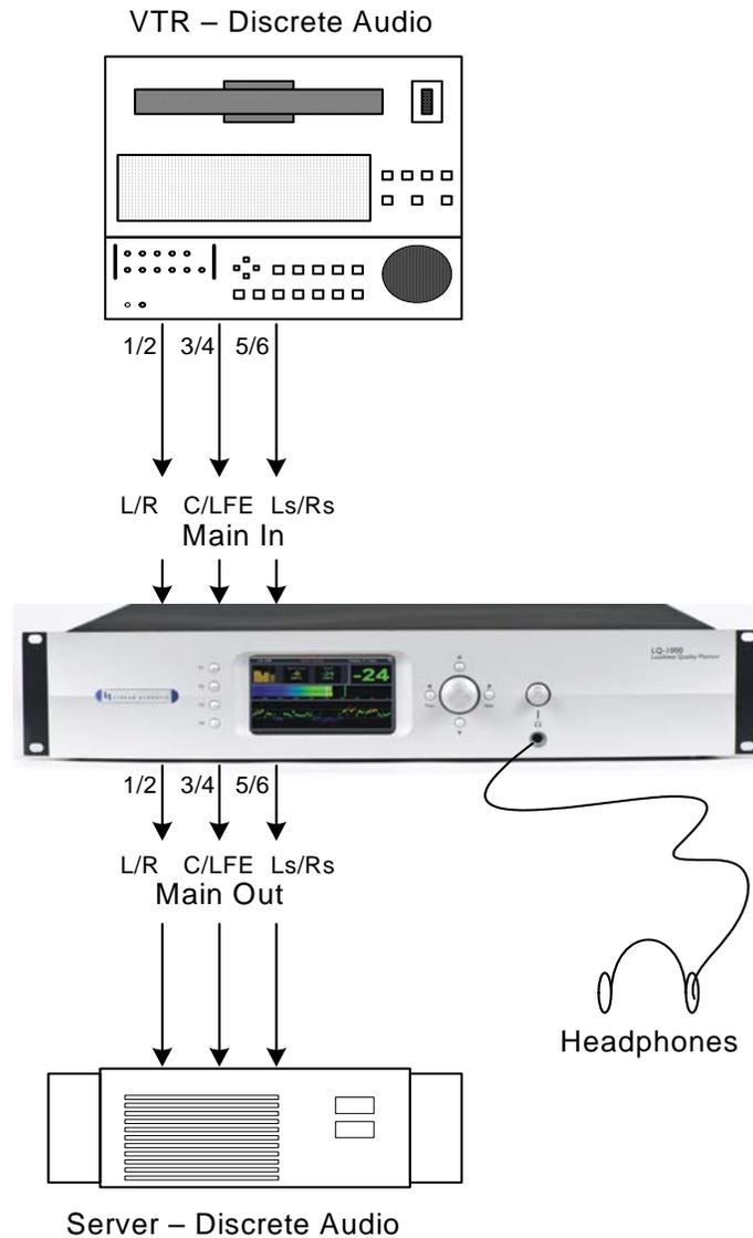
**Figure 3-6** LQ-1000 Used for ingest of discrete audio channels
