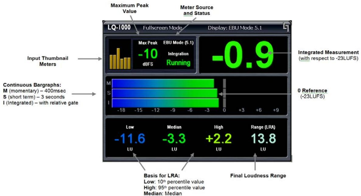
Figure 3-4 EBU Mode screen for channels 1-6
