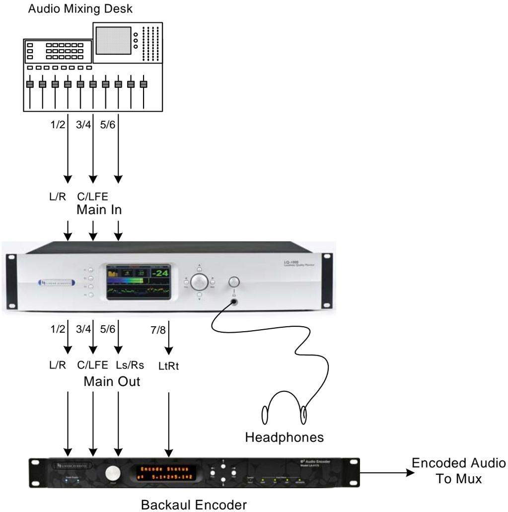
**Figure 3-9** LQ-1000 used for live production
