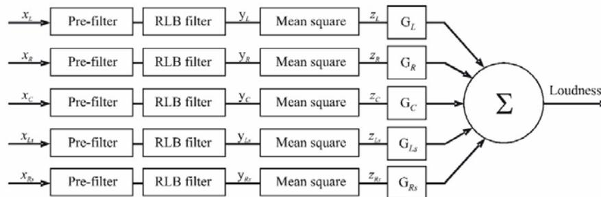
**Figure 3-1** Block diagram of ITU-R BS.1770 multichannel loudness algorithm
