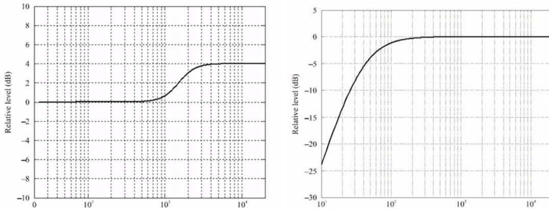
**Figure 3-2** Responses of the pre-filter to account for acoustic effects of the head (left), and the RLB high-pass filter (right) combine to produce the so-called K-weighting filter.
