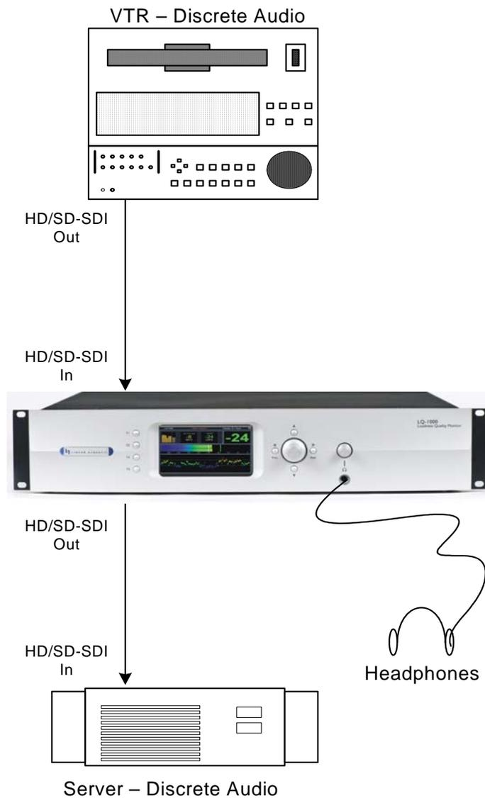
**Figure 3-7** LQ-1000 Used for ingest of SDI embedded audio channels
