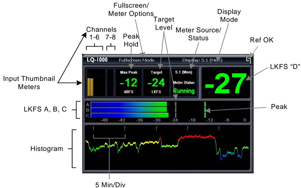
**Figure 3-3** Fullscreen ITU mode display for channels 1-6
