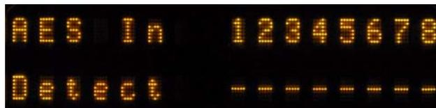
Figure 4-6 AES presence detect for applied pairs (1-4 are used)
