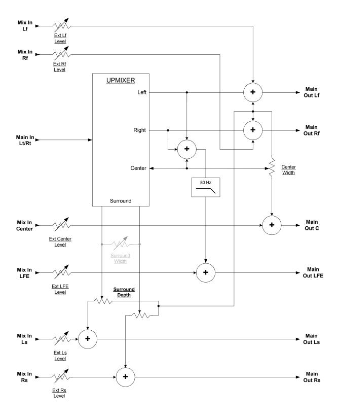
Figure 1-1 Audio Block Diagram
