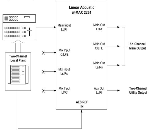
Figure 3-1 UPMAX 2251 in a commercial upmixing application
