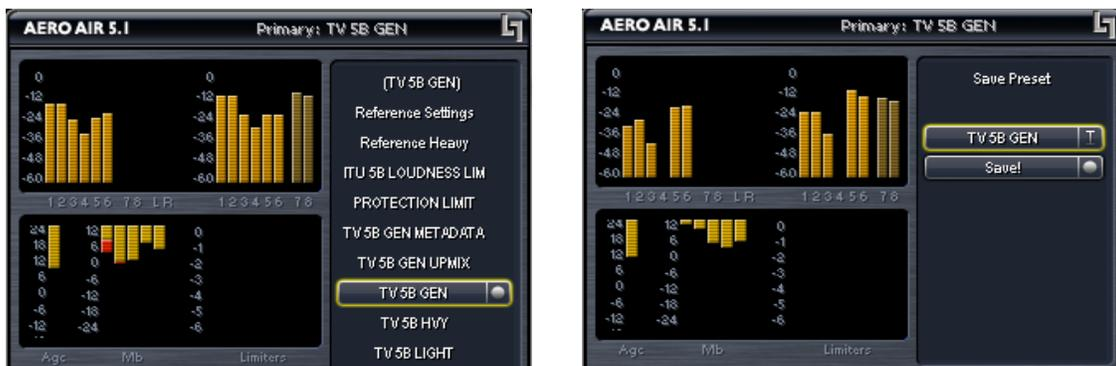
Figure 4-2 Recall Preset menu (left) and Save Preset menu (right)
