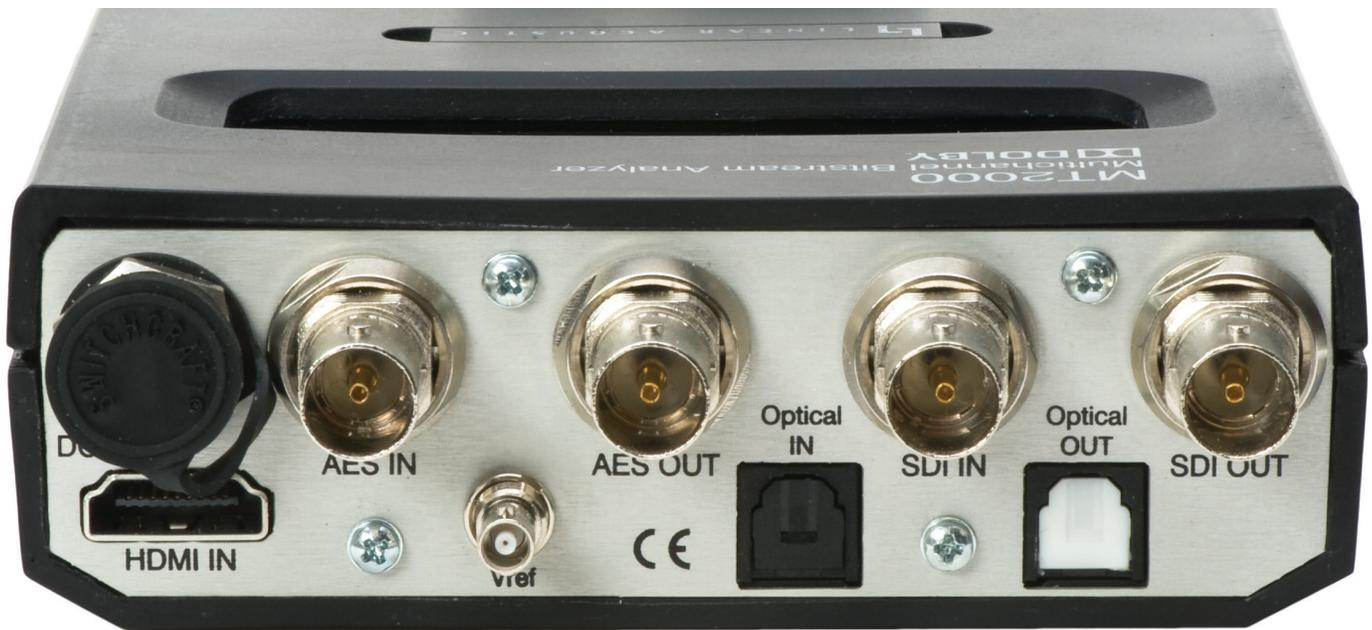
The Linear Acoustic MT2000 Bitstream Analyzer is a portable, handheld diagnostic tool that can monitor and generate Dolby Digital, Dolby Digital Plus, Dolby E, and PCM bitstreams.
