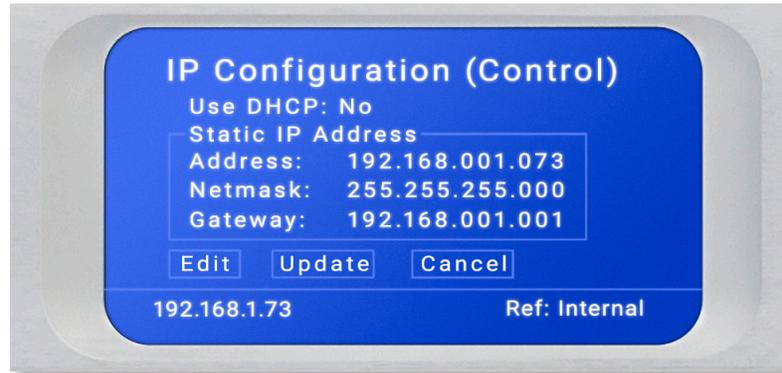
Figure 4-5 – Front panel IP configuration screen
