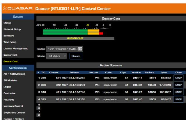
Included as part of the Quasar Soft license, **Quasar Cast** is a remote monitoring solution that lets you listen to any Livewire stream in the network through the same web browser. Quasar Cast generates a compressed OPUS stream from a source in the Livewire® network and can serve up to eight clients (including Quasar Soft instances). With Quasar Cast, you can listen to what is happening in the studio, and on the air, while you operate the console remotely using Quasar Soft.
