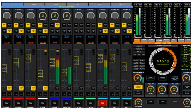
**Quasar Soft** is a customizable remote control solution that lets you control the Quasar surface from your browser. You can generate up to eight HTML-5 pages and configure them to display any of the 64 input channels, plus a small monitor section, or even the entire master section of the console. Quasar Soft comes standard with Quasar XR consoles and is an optional upgrade for Quasar SR consoles.
