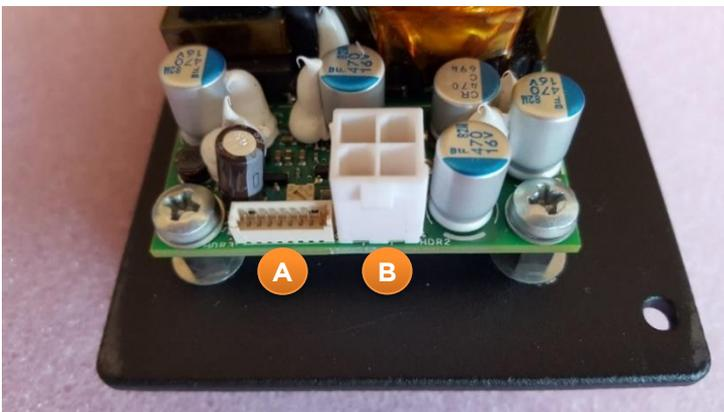
These are wired to the corresponding 1-4 inputs of the power distribution board. The Power distribution board outputs 12VDC power to the modules, and actively controls load sharing between the installed Power Supplies.
