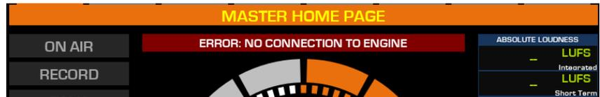
If frequent or random loss of connection is experienced, and the **Switch Statistics** page reports a high quantity of Tx/Rx errors, you may have problems with your Ethernet wiring and more specifically, with its grounding. Please see Chapter 2 - [Earth Connection and Grounding](#).
