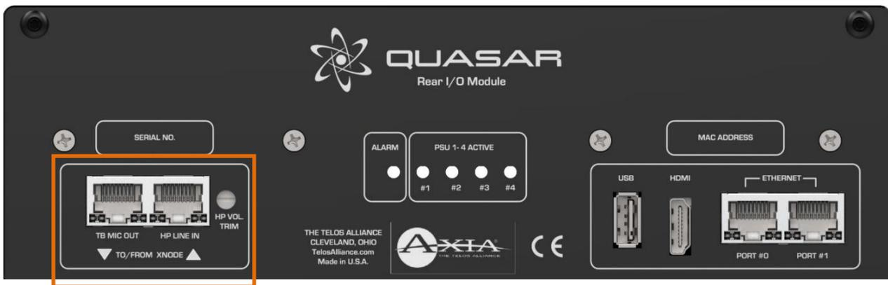
Connect the TB MIC OUT (A) socket to the input of your xNode , and the HP LINE IN socket to one of the outputs of your xNode using standard RJ-45 cables.
