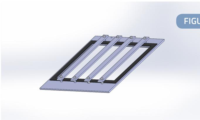
4. Remove the 8 - 5.5 mm nuts that hold the 4 retention bars in place, and the retention bars.
