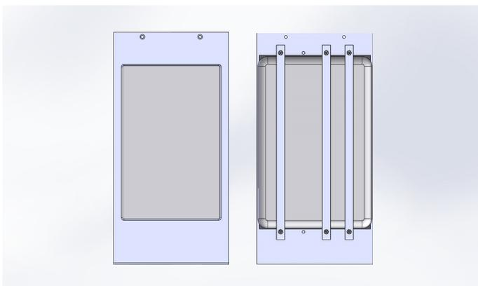
8. With your Tablet installed safely, do a quick press test to make sure it does not move. If it does, tighten the nuts slowly till it no longer shifts.
