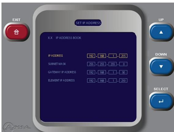
To quickly configure the Timer, touch and hold the red **RESET** control on the timer screen. After 5 seconds, the IP Address Book Screen will appear. This screen is where you'll set the Timer's own IP address, and tell it which Element to work with.
