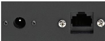
Connect a CAT-6 Ethernet cable between the Timer and the local Axia network switch, using the RJ-45 port on the reverse of the unit.
