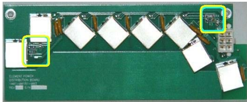
Figure 1 (Revision 2 Power Distribution Board)
