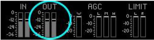
Processing adjustments will be heard real-time on local outputs, but will be heard with a certain amount of delay in the encoded stream. A small portion of this delay is introduced by the encoder while a much larger portion is introduced by buffering in the server and the client used to listen to the stream.
