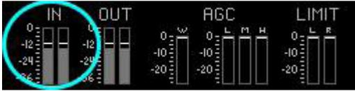
Increase INPUT gain by pressing the encoder knob, turning, and then pressing again to set the value.
