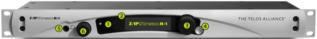
1. **Power LED:** The blue power LED is located to the upper left of the display. When the unit is first powered, the power LED will flash until the unit is fully booted. When booted, the power LED will light solid.
