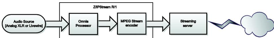
This section walks you through a simple setup where the Z/IPStream R/1 is fed analog audio, the network settings are configured via DHCP, and the stream is sent to a ShoutCAST v2 server. If your setup is different, you may safely skip this section. If this is the first time you have used a Z/IPStream R/1, you may want to have a look at the [Front Panel] and [Entering Text] sections in the back before you proceed.
