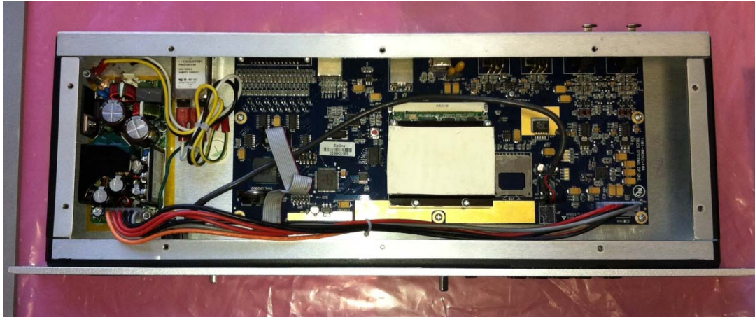
Figure 3: completed cable replacement
