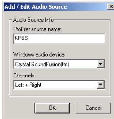
3. Select the desired Windows audio device then enter a descriptive name in the *ProFiler source name* field.
