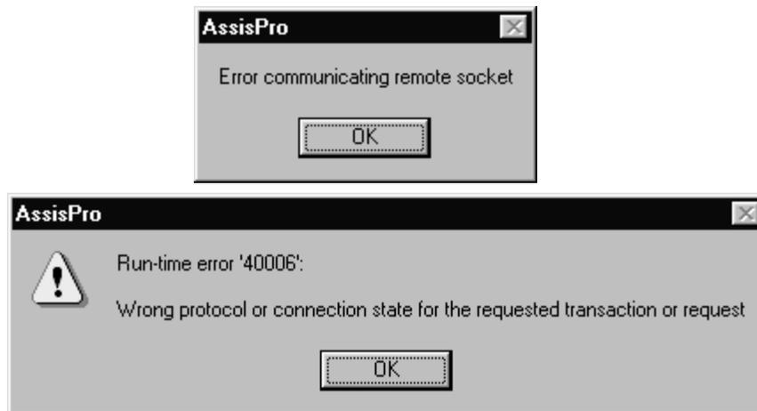
The above errors are produced by either a failure in the Server PC, no network connection, or Incorrect IP address.
