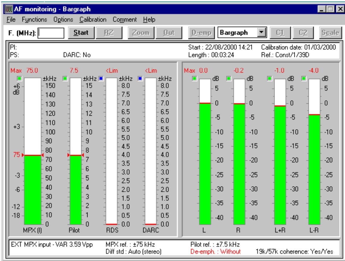
Peak Measurement Of MPX Signal With Omnia.fm Processor
