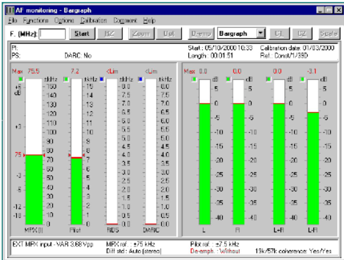
*Peak Measurement Of MPX Signal With Orban 8400 Processor*
