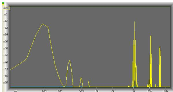
Figure-9, Clipper Induced IMD: 100Hz & 5kHz
