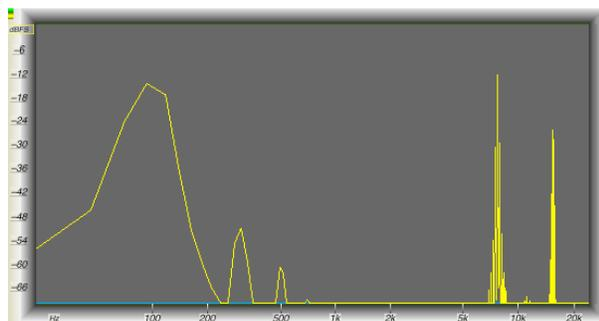
Figure-10, Clipper Induced IMD: 100Hz & 7.5kHz
