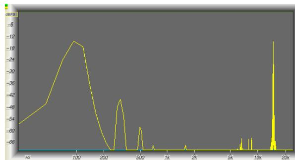
Figure-13, Clipper Induced IMD: 100Hz & 15kHz
