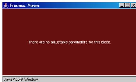
In Omnia 8x's implementation, the crossover network is carefully time-aligned so that the recombined spectrum remains flat, regardless of the amount of gain control being applied within any band. This true phase linear response assures that harmonic overtones are not displaced in time. The result: the truer, more natural, and more musical Omnia sound. The crossover frequencies are not adjustable.
