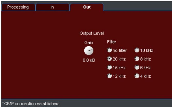
Peak *Output Level* adjustment is done using the single *Gain* control that adjusts both the Left & Right channels together. The control range is from -26dB to +6dB of gain. This level is normally set to the maximum input level, or just below it, of the device that the Omnia 8x output is connected to.
