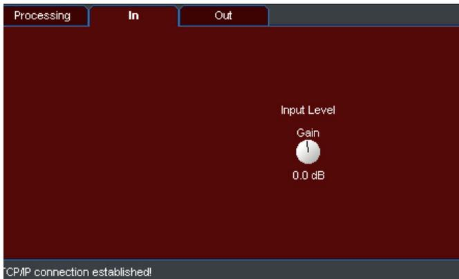
Click on the knob to highlight it and adjust the mouse wheel (if present) or click-hold and move the mouse itself left or right to adjust the level. There is a 30dB range of adjustment between -20dB and +10dB.
