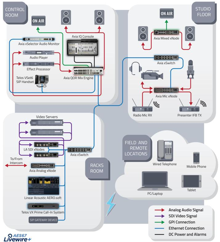
Telos, Axia and Linear Acoustic Audio-over-IP products combine to create a comprehensive TV Studio audio system aimed at the cost conscious client who demands a best-of-breed solution. Designed without compromise, an AoIP facility based around the Livewire+/AES67 standard, can evolve along with the broadcasters most exacting demands and expectations using the unparalleled flexibility of IP.
