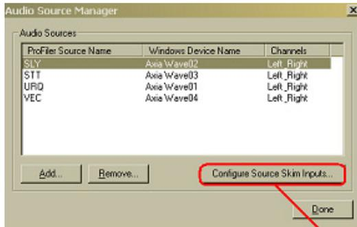
The iProFiler Setup screen has a button labeled “Audio Sources...”. This button brings up the Audio Source Manager (shown above). The manager allows for the creation of sources as well as the ability to configure Skimmer control (GPIO Configuration).
