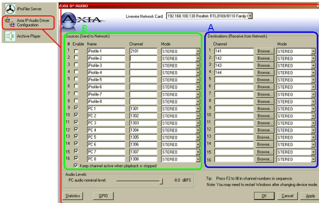
iProFiler accepts as sources the 16 "Destinations" (Receive from Network) fields. In these fields (marked "A" above), you select the channel numbers that you wish to record.
