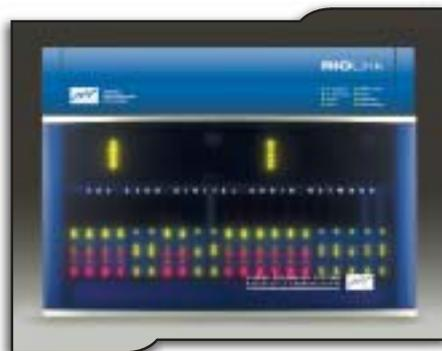
The RIOLink (top) from SAS provides remote I/O connectivity for the 32KD Digital Audio Network (bottom) via CAT-5 or fiber optic cabling.
