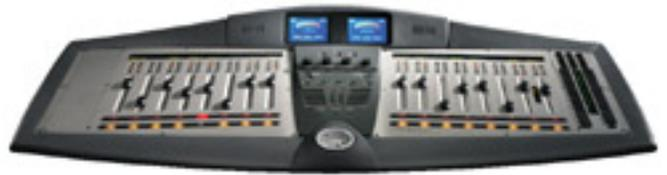
The **Harris BMX Digital** is an all-digital design that features 48 digital buses that can be configured for program mixes and talkback channels. It has four program buses, four utility buses and two send buses, each with analog and digital outputs. It supports as many as six telco modules with their own off-line mixes, with two additional off-line mixes for other mix-minus uses.
