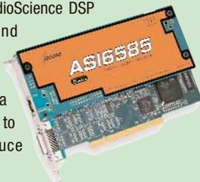
Using a powerful Texas Instruments onboard floating point DSP with Axia Livewire networked audio protocol allows the AS16585 to simultaneously play up to eight stereo streams of audio which can be mixed to eight stereo outputs, and record up to eight audio streams fed from eight stereo inputs, over switched Ethernet. The feature set of the AS16585 extends to MRX multi-rate mixing, MPEG Layer 2 and 3 encoding and decoding, TSX time scaling and SSX2 multichannel record and playback.
