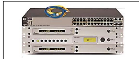
A small (16x16 stereo) routing switcher configuration.
