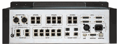
The rear panel of PowerStation showing microphone inputs, analog and AES inputs & outputs, GPIO ports and multiple Ethernet expansion ports.
