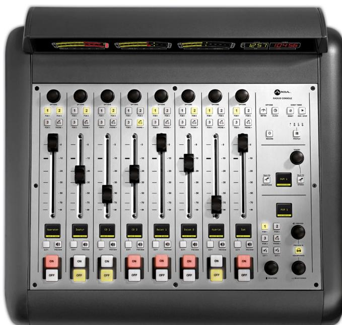
There are also OLED displays on every fader that provide source assignments, pan & balance settings, fader options and more — which means no additional computer monitors or mice to clutter up your studio. The display can also work with the Soft Keys just below to trigger GPIO events, step automation events, and adjust source input options.
